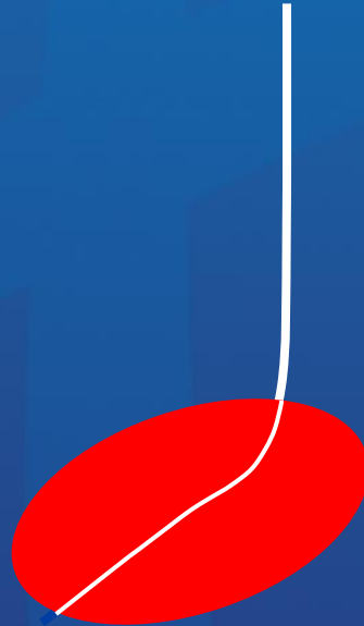
Wellbore Azimuth Parallel To Fracture Azimuth
