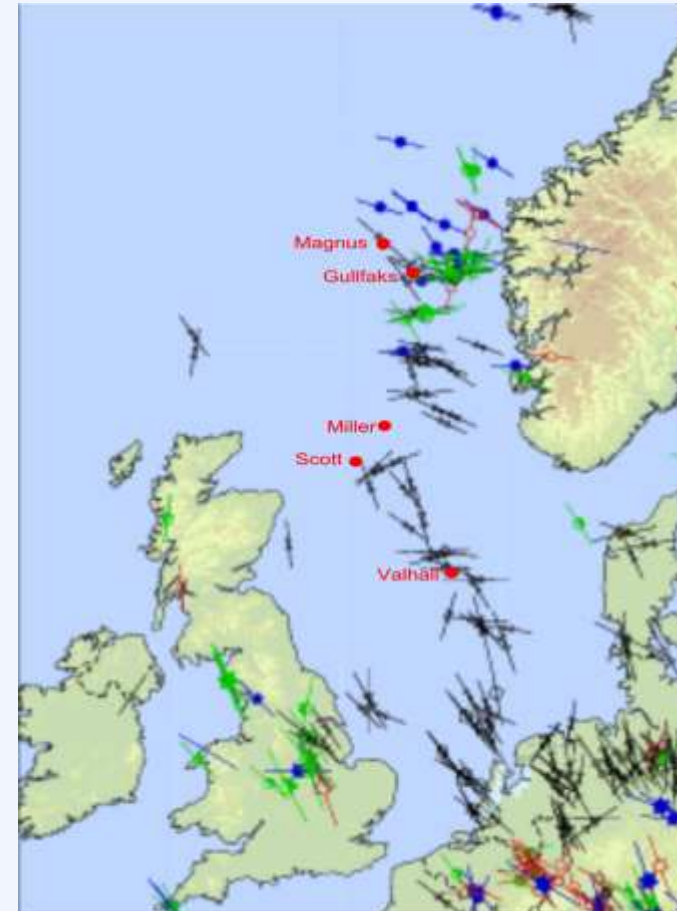
Maximum horizontal stress axes (World Stress Map Heidbach et al (2008))
